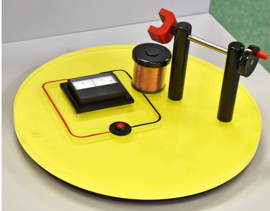
**Can you make an electric current by moving the magnet near the coil?**
